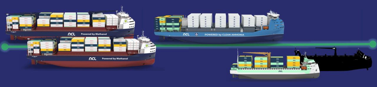
1<sup>st</sup> - MeOH vessel 2<sup>nd</sup> - MeOH vessel NH3 vessel 250 TEU NH3 Shuttle 2 x 150 TEU Battery Shuttle
