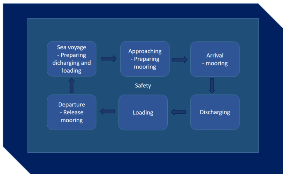
Figure 1 – Simplified process of main activities of a port call for a merchant vessel.
