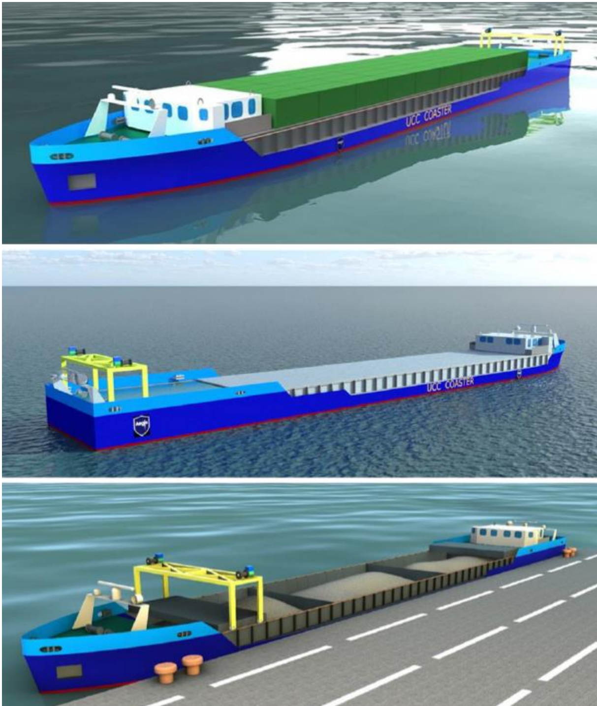
Figure 4 – ISE concept for a low-emission autonomous shallow water coaster. From: AEGIS, 2023a[13]
