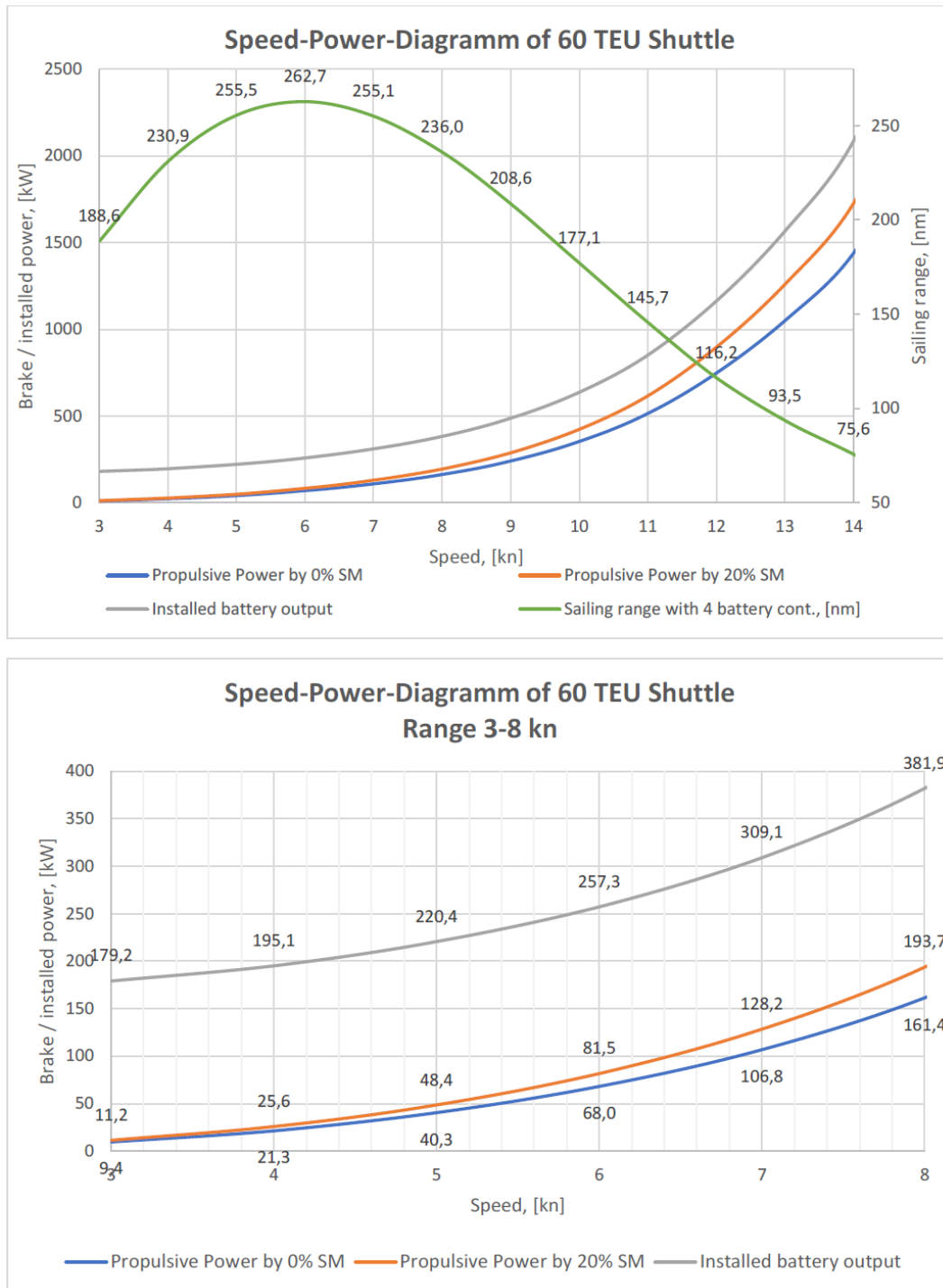
Figure 10: Use Case A, speed-power diagram of daughter vessel. Source: ISE.
