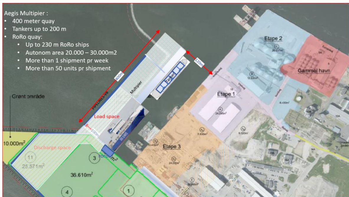
Figure 3 – First design AEGIS multi pier
